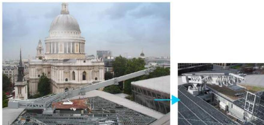
Figure 8. Example: BMU capable of parking below roof (Source: Cox Gomyl)
